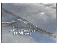
**Step 12**- Using a compressed air source, test all bonded seams using a minimum 50 p.s.i. (344.74 kPa) air supply directed through a 0.1875" (.48 cm) nozzle held within 2.00" (5.08 cm) of the seam edge.
